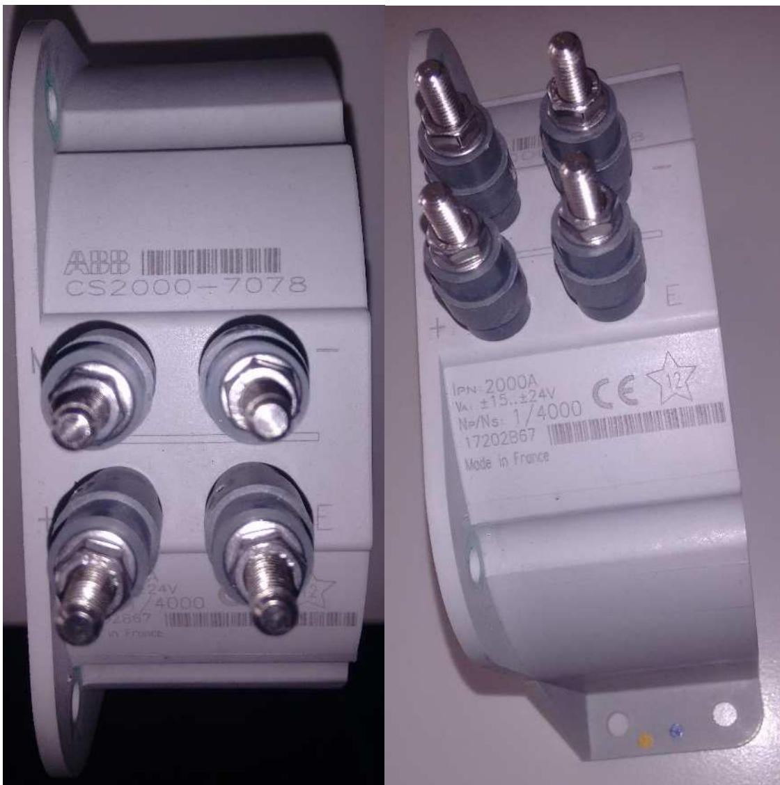
Figure 24: type plate of previously used current transducer CS2000-7078
